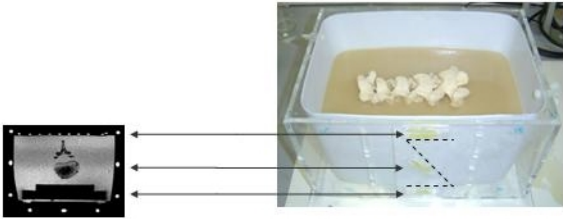
Figure 2.17: Phantom design showing human cadaver spine partially embedded in tissue equivalent gel. Fiducial markers are shown both on the phantom and the corresponding MR image.
