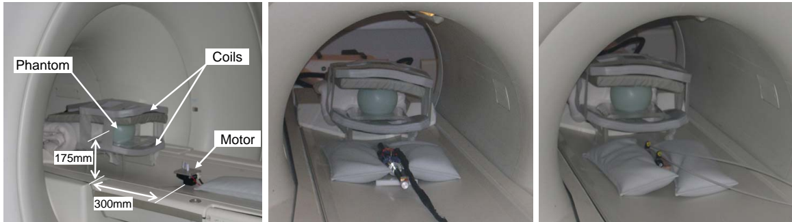
Figure 3.6: General experimental setup for compatibility test in 1.5T MR scanner with Shinsei motor (left), Nanomotion motor (center) and Pneumatic cylinder (right).
