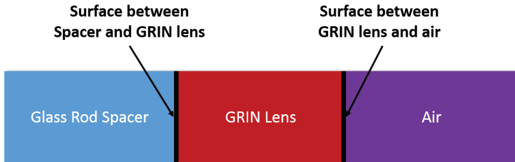
Figure 7.2. An abstract model of the distal end of the OCT imaging probe that consists of three optical components and two optical surfaces as described.
