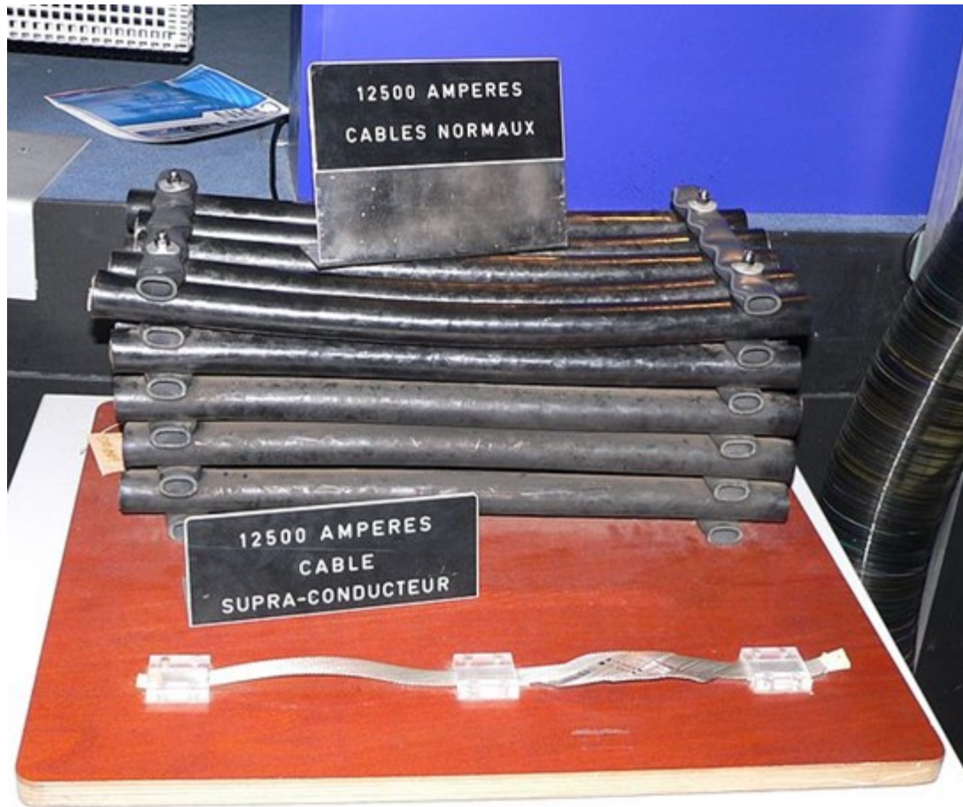
Figure 7.1. Conventional electrical cables and superconducting cables used in accelerators at CERN (Wikimedia 2017)
