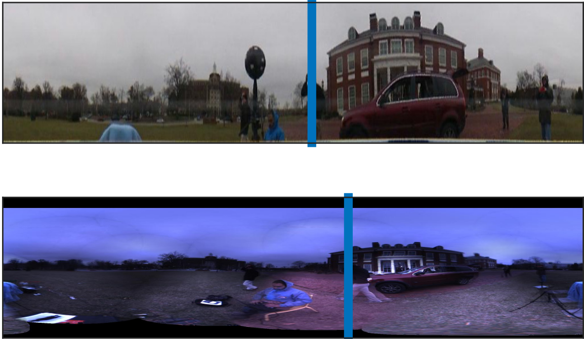
Figure 7.9: Localization results for both the VisiSonics system and the combined Bloggie camera/Eigenmike system. The panel on top is from the combined system, and the panel on the bottom is from the VisiSonics system. The blue lines indicate the localized angles calculated using only the raw microphone data from each system. This particular frame of the video illustrates the differing perspectives of the two cameras and shows why the angles in Figure 7.8 do not exactly match.
