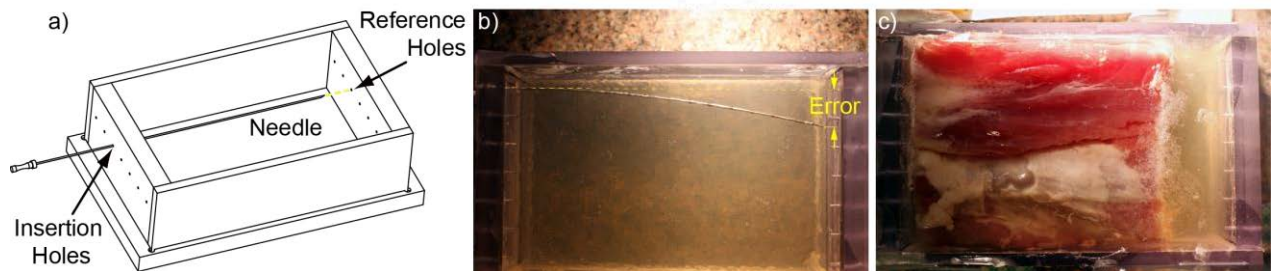
Figure 37: The setup: a) experiment box and b) targeting error measurement example, c) box with ex-vivo tissues fixed in gelatin (deepest side clear for measurements).
