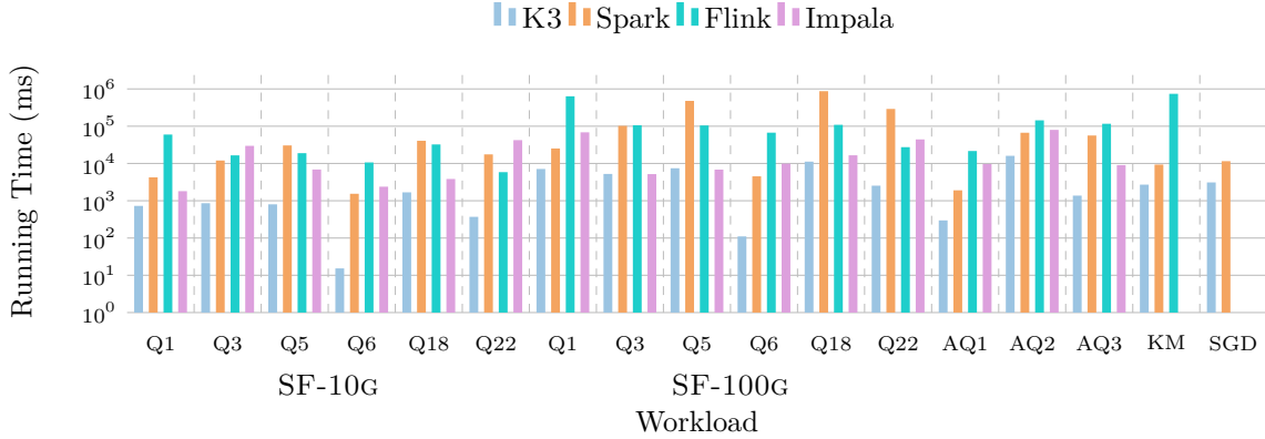
Figure 5.4: End-to-end running-time comparison of K3 against Flink, Spark (2.0.1) and Impala scheme using almost entirely references for both loop and accumulator variables — each optimization eliminating the allocation of an entire class of intermediate data. Furthermore, the accumulator in Q6 is a single statically-sized integer, and is therefore inferred to be stack allocatable in K3. Apart from K3, only the newest version of Spark is able to take advantage of this property, in the simplest case of Q6.
