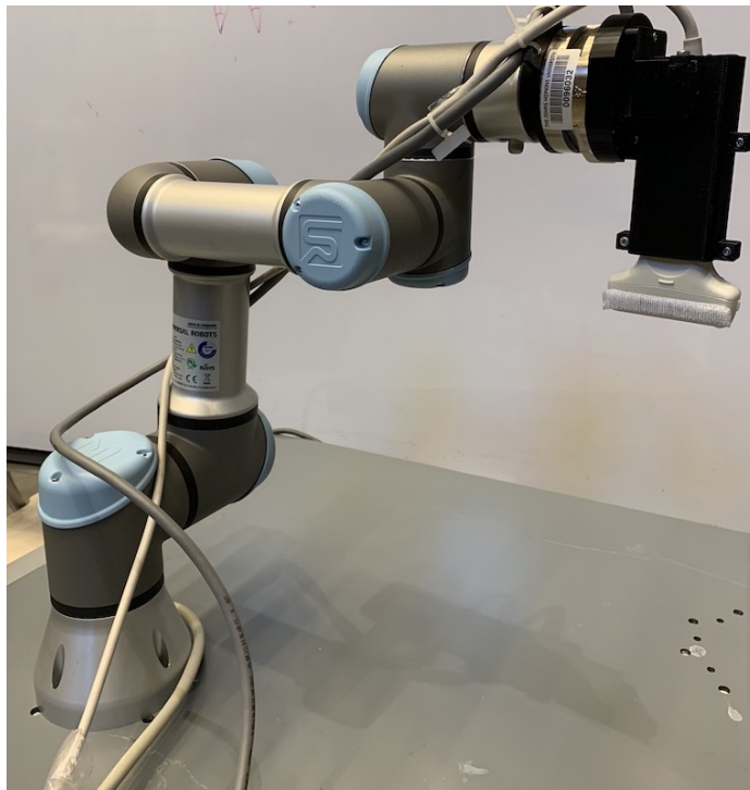
Figure 6.9: UR3 robot with an ultrasound transducer attached to the end-effector
