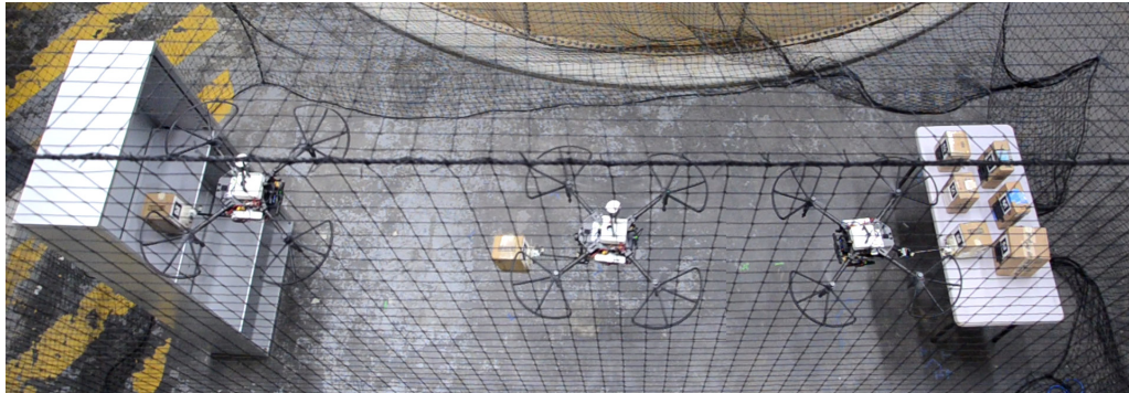
Figure 6.8: Time-lapse of the aerial manipulator picking the object highlighted in yellow from the packaging area (top-left) and placing it on a storage shelf (top-right) in the same trial. The bottom picture shows an overhead view of the pick-and-place procedure.
