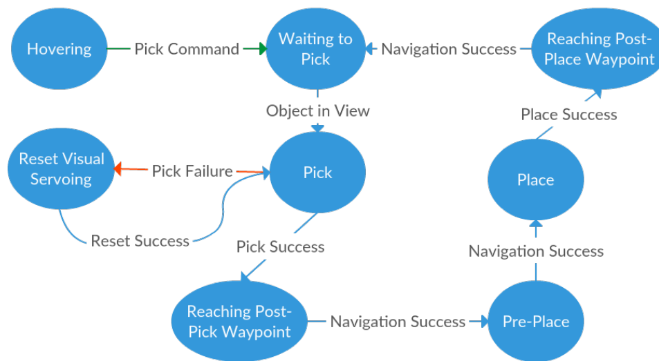
Figure 6.9: Part of the state machine for picking and placing a package. The recovery actions are red and user actions are green. The user can also abort from any other state back to hovering if manual intervention is desired.
