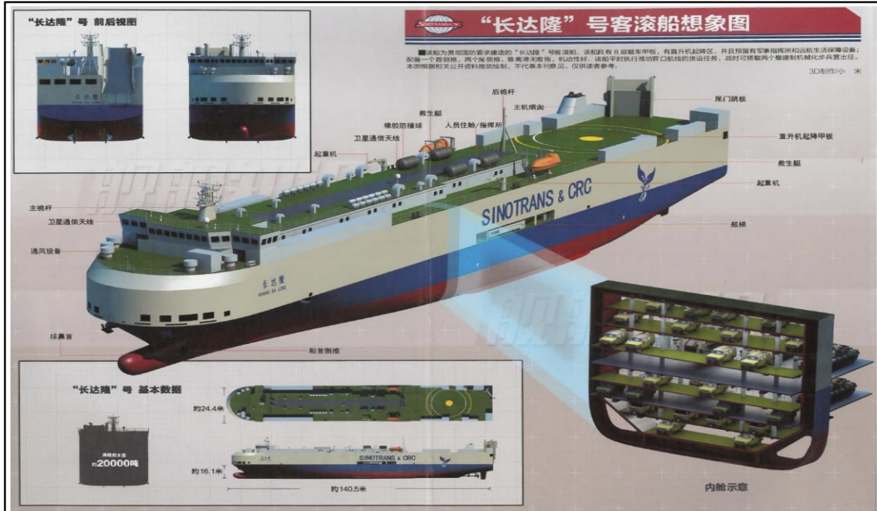
Image 3.2: Naval Ships and Merchant Magazine depiction of Roll-on-Roll-off vessels for vehicle transport. 43
