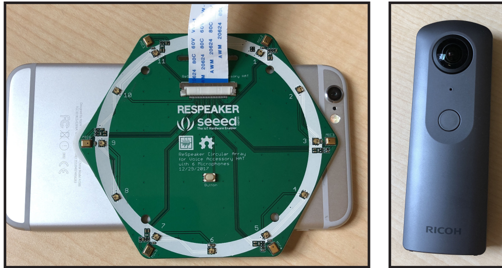
Figure 2.2: Audiovisual zooming is implemented on two mobile platforms: an off-the-shelf planar microphone array (with 6 microphones) is attached to a smartphone [left] and a 360° Ricoh camera [right] to show smartphone and teleconferencing utility.
