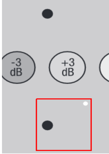
Figure 4.2: Schematic diagram of phantom used for the plane wave data. The red rectangle shows the anechoic target of interest for our study.
