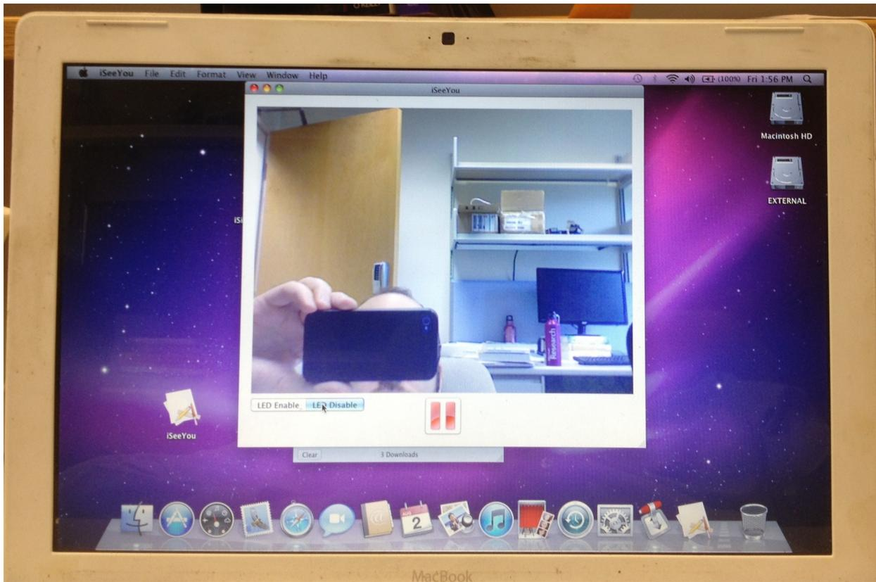
Fig. 3: *iSeeYou* running on a white MacBook “Core 2 Duo” capturing video from the internal iSight with the LED (the black dot to the right of the square camera at the top, center of the display bezel) unilluminated.
