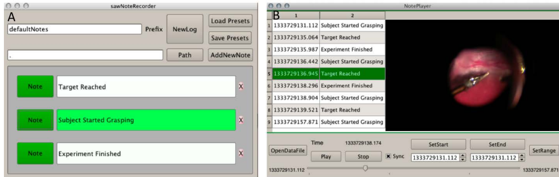
Figure 3.15: A) Note Recorder application. B) Note Player showing video frame corresponding to a note.
