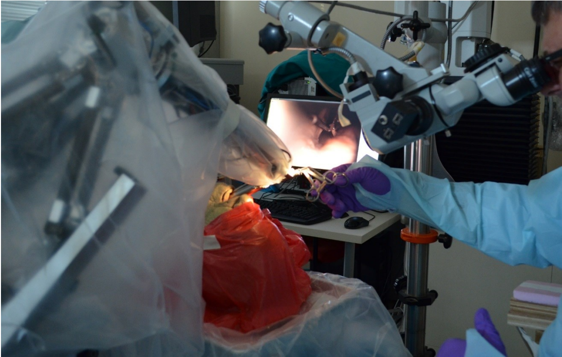
Figure 4.20: Hands-free tissue holding with REMS.
