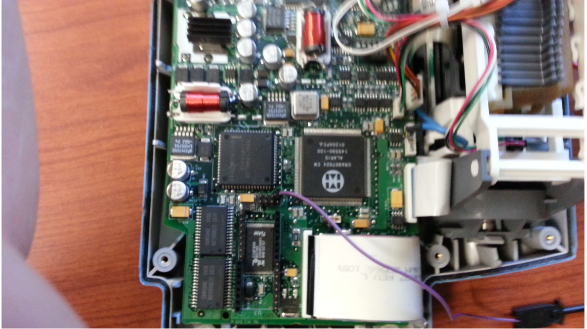
Figure 4.3: Board Layout of the Alaris SE 7132. Redundant SRAM chips on left, CPU top-middle, flash between header pins, ASIC top-right.
