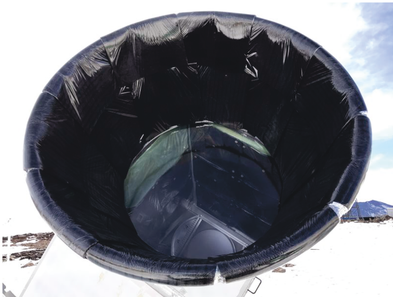
Figure 5.13: Forebaffle blackening. The forebaffle was blackened with ECCOSORB HR-10 sheets in bags, which were firmly fixed to the forebaffle. The blackening increases detector loading by < 0.1 pW.
