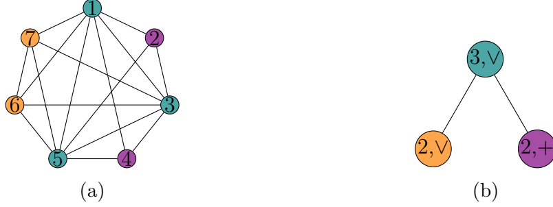
Figure 4.1: (a): A cograph given by C = (\mathbf{1} \vee \mathbf{3} \vee \mathbf{5}) \vee (\mathbf{2} + \mathbf{4} + \mathbf{7} \vee \mathbf{6}) . (b) The twin reduction graph R_C . The vertex labels are the twin numbers and the types of the twin classes.
