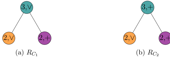
Figure 4.2: (a): Twin reduction graph of a cograph given by C_1 = (\mathbf{1} \vee \mathbf{3} \vee \mathbf{5}) \vee (\mathbf{2} + \mathbf{4} + \mathbf{7} \vee \mathbf{6}) with spectrum \Lambda(C_1) = \{0, 3, 3, 5, 7, 7, 7\} . (b): Twin reduction graph of a cograph given by C_2 = (\mathbf{1} + \mathbf{3} + \mathbf{5}) \vee (\mathbf{2} + \mathbf{4} + \mathbf{7} \vee \mathbf{6}) with spectrum \Lambda(C_2) = \{0, 3, 3, 4, 4, 5, 7\} . Note that \Lambda(C_1) and \Lambda(C_2) have five eigenvalues in common, as predicted by Conjecture 4.3.
