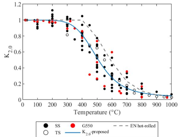
Figure 8: Comparison of proposed retention factors for 2.0% stress.
