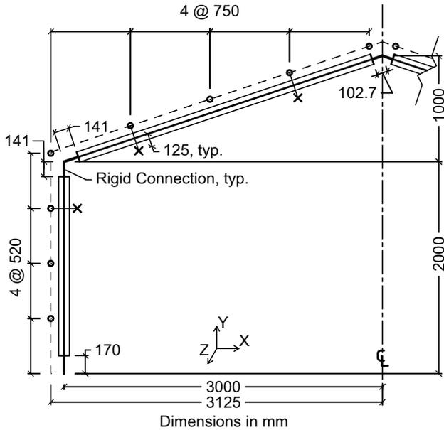
Figure 1: Single channel portal frame geometry. Dimensions shown are symmetric
