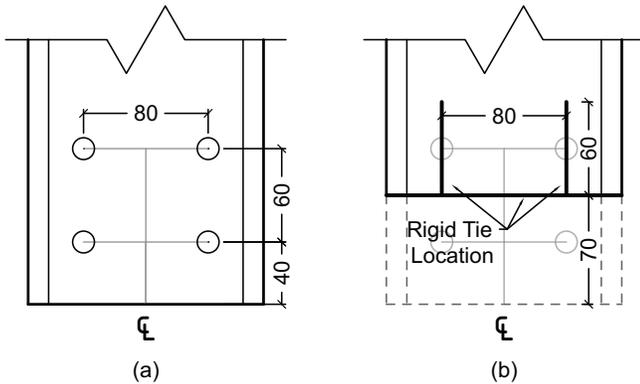
Figure 4: Dimensions of channel (a) end bolted connection and (b) rigid tie model
