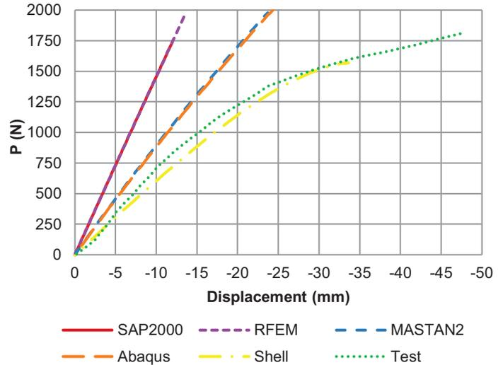
Figure 5: Vertical displacement at midspan of left rafter for Load Case 1
