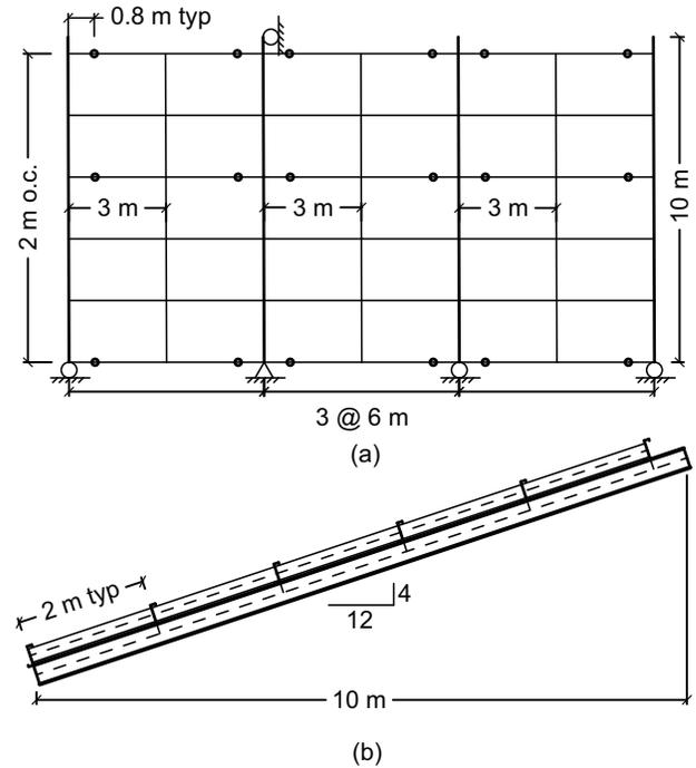
Figure 6: Roof layout (a) Plan view (b) Section view
