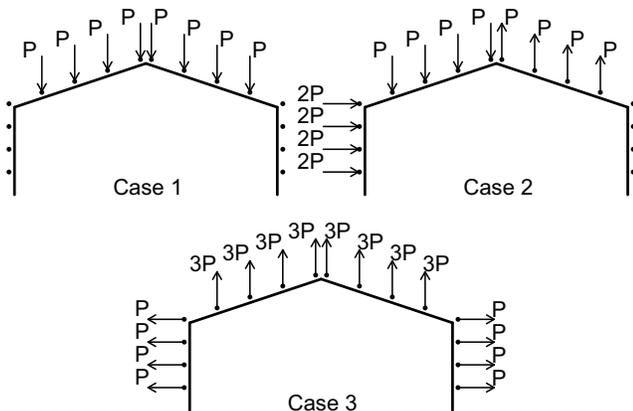
Figure 2: Three loading scenarios applied to portal frame
