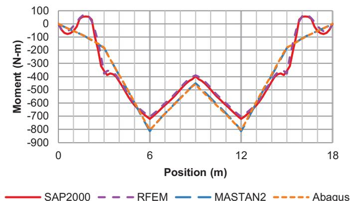
Figure 8: Geometric weak axis moment from uplift loading along 4th purlin. Position = 0 is the left side of Figure 6a
