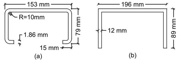
Figure 3: Cross-sectional dimensions of (a) lipped channel and (b) bracket
