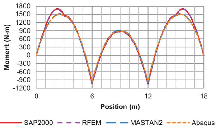
Figure 7: Geometric weak axis moment from vertical loading along 4th purlin. Position = 0 is the left side of Figure 6a
