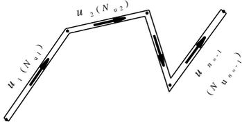
Fig. 6 Transverse displacements of GD modes
