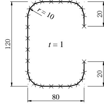
Fig. 4 A lipped channel with rounded corners
