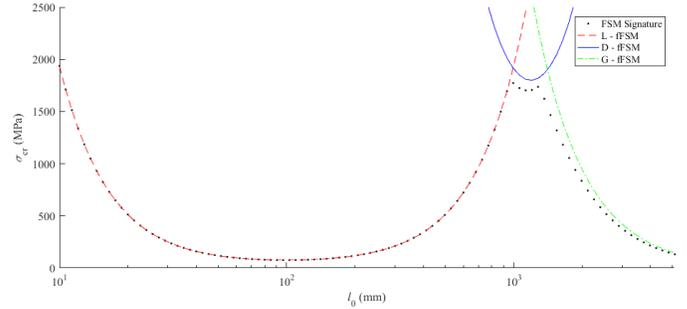
Fig. 11 Modal decomposition of the square steel tube under axial loading
