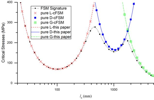
Fig. 3 Modal decomposition of a lipped channel under axial loading
