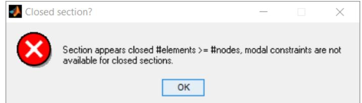
Fig. 9 Classic cFSM not able to handle closed cross sections
