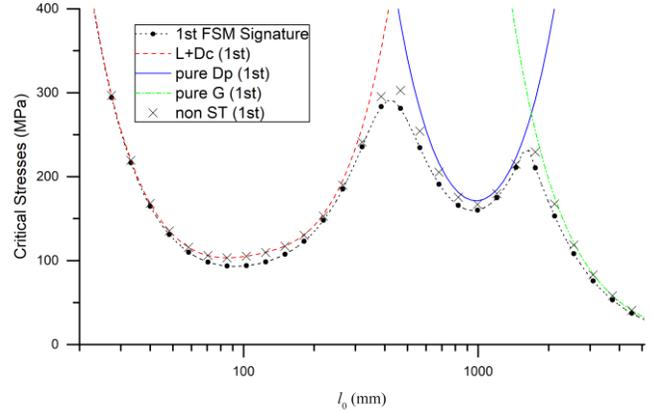
Fig. 8 Modal decomposition of rounded corner sections under axial loading
