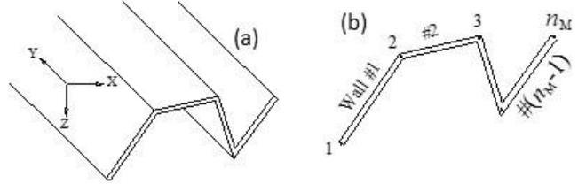
Fig. 1 (a) A thin-walled member and (b) the main nodes and plate elements
