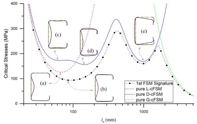
Fig. 5 Mode decomposition of a lipped channel with rounded corner under axial loading
