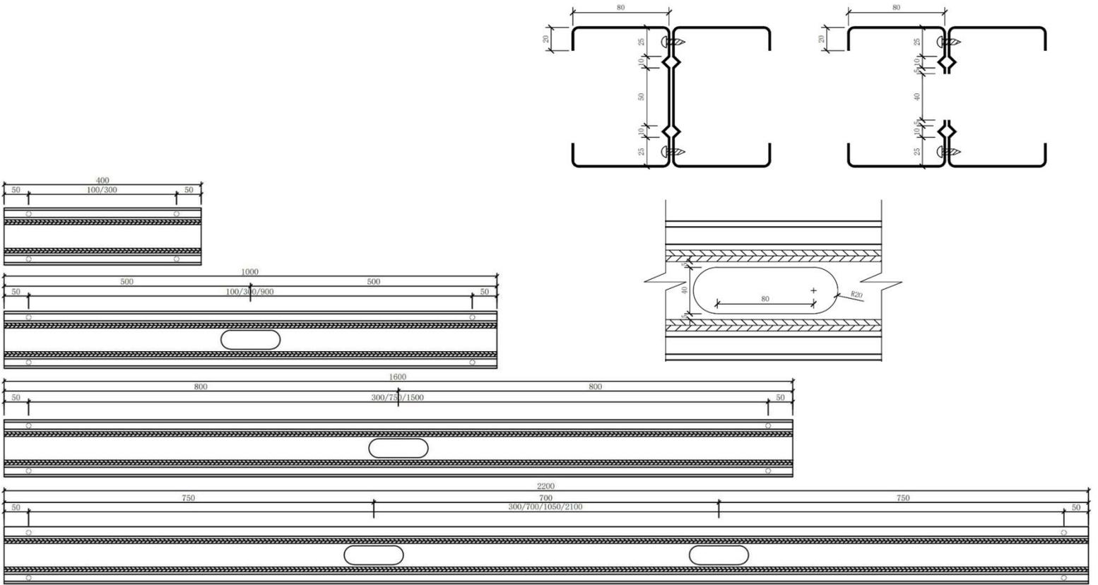
Figure 2 C-shaped cross-section split H-shaped bending member
