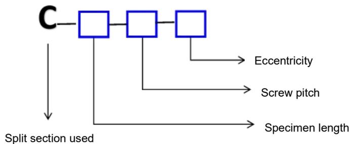
Figure 1 Numbering rules of test pieces
