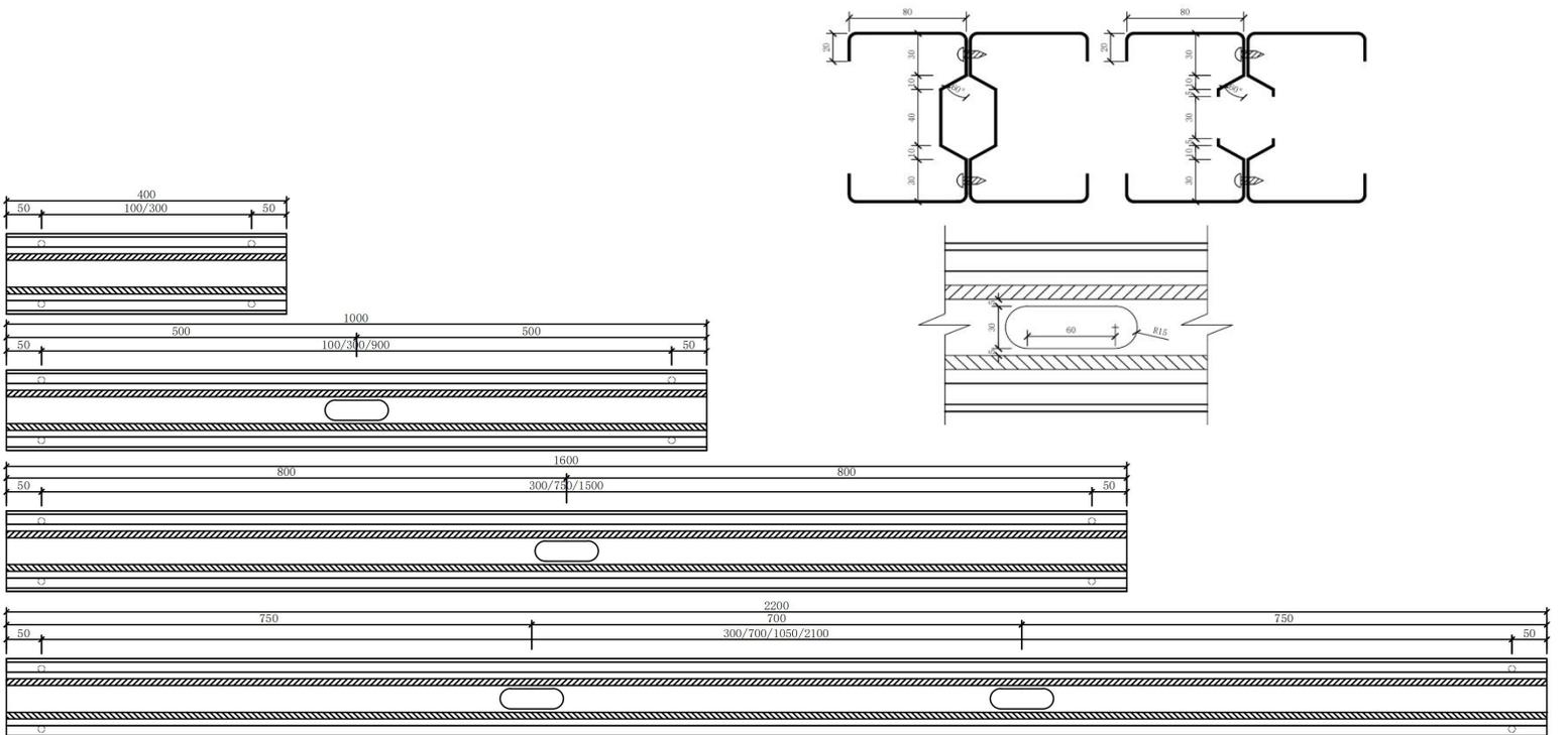
Figure 3  $\Sigma$ -shaped section split H-shaped bending member
