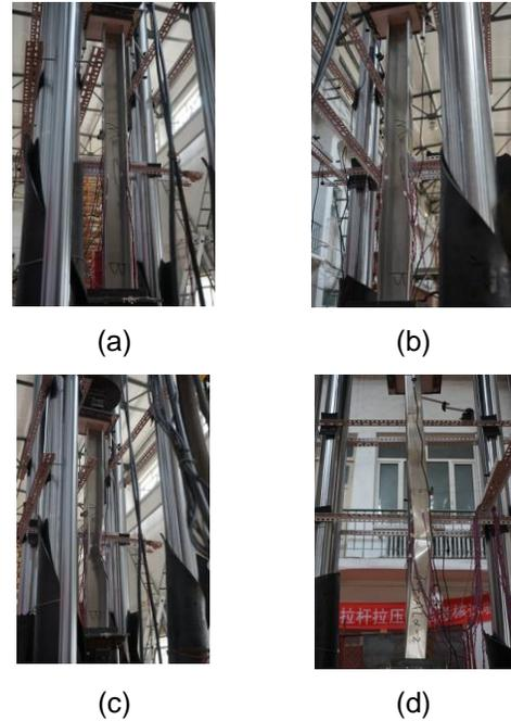
**Fig.8** Loading process of specimen 304-AL $\alpha$ -2
