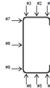
(a) Measurement points of cross section
