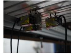
(c) Grooves and laser displacement meter
