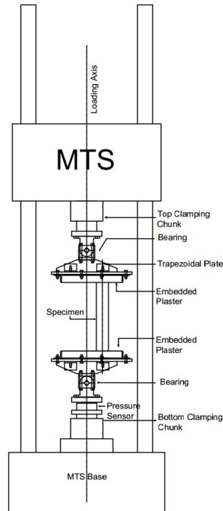
(b) Side elevation of test set-up
