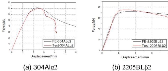
**Fig.12** Comparisons of force-displacement curves
