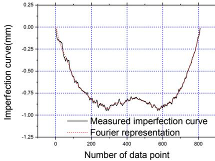
Fig.5 #1 measurement line imperfection curve of 304-AL $\alpha$ -1 member
