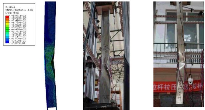
**Fig.11** Buckling deformation
