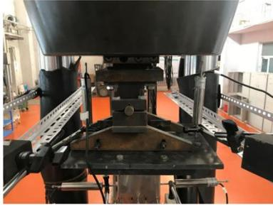
**Fig.7** Bearing and trapezoidal plate
