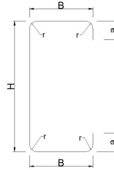
Fig.1 Nomenclature for C section dimensions
